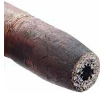
Nozzle fully clogged (not using E-WELD Nozzle)
