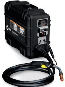
Easy solution for traditional wire process. Add the flux-cored capability of the PipeWorx 350 FieldPro™ for fill and cap passes for increased productivity.
