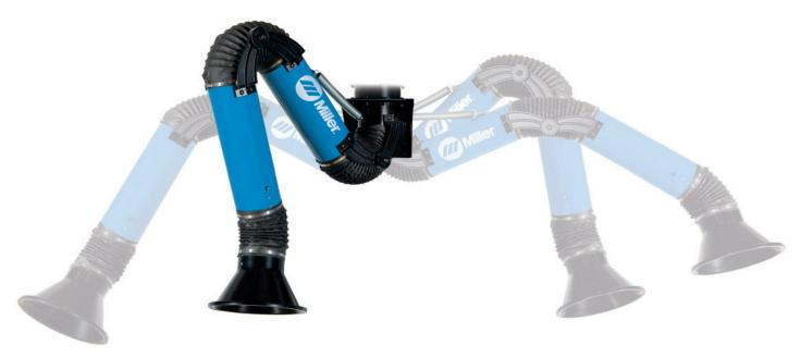
**Easy-to-operate standard arm** has external adjustments so air can pass through with less airflow resistance, giving you stronger cfm (airflow). It offers reliable and accurate positioning across the full range of motion, as well as easy adjustment and maintenance to ensure long-lasting operation. Pre-assembled extraction arms are available in 7-, 10- or 12-foot lengths.
