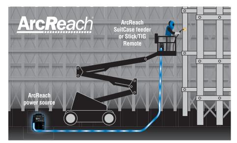
**Remote control of the power source without a cord.** ArcReach technology uses the existing weld cable to communicate welding control information between the feeder or remote and the power source. This technology eliminates the need for control cords, and their associated problems and costs.
