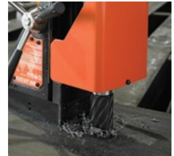
For larger hole, 1/2" and above, use magnetic base with standard Weldon shank
