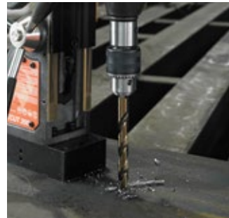
Includes a 1/2" chuck adaptor for small hole drilling
