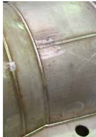
Seawater pump in UNS S32205 duplex stainless steel welded using Avesta FCW 2507/P100-PW (E2594T1-4/1) for highest possible corrosion resistance.
