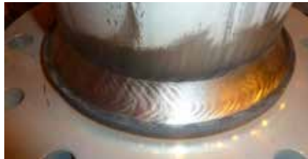
Fillet weld in flat position (PB / 2F). The base material is AISI 304L and the filler Avesta FCW-2D 308L/MVR (E308LT0-4/1). Ø1.2 mm (.045").
