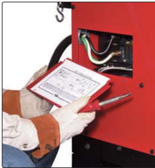
Easily accessible input voltage reconnect panel.
