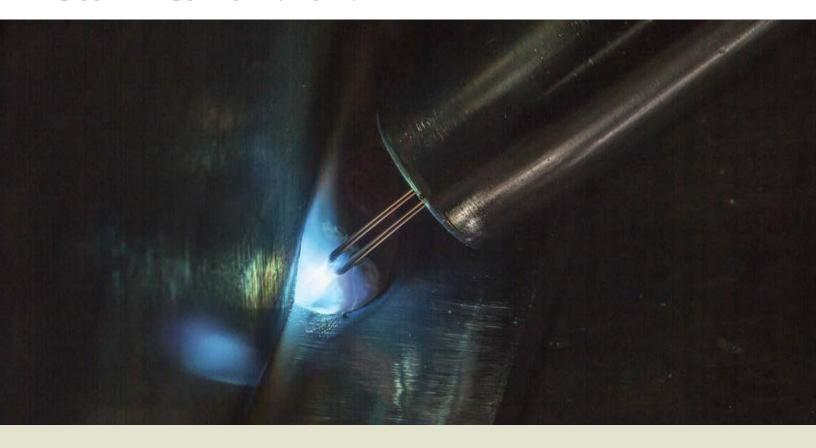
The HyperFill™ twin-wire MIG solution was developed to revolutionize heavy fabrication productivity. Designed for semiautomatic and robotic applications, HyperFill redefines high deposition welding — allowing you to make larger welds, faster and more easily. With its innovative twin-wire design, HyperFill allows for deposition rates above 18 lbs/hr (24+ lbs/hr robotically) without compromising weld quality or operator ease-of-use.
