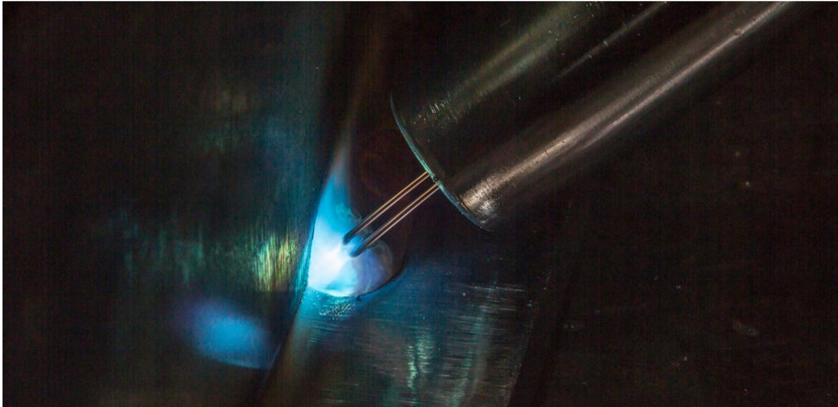
The HyperFill® twin-wire MIG solution was developed to revolutionize heavy fabrication productivity. Designed for semiautomatic and robotic applications, HyperFill redefines high deposition welding – allowing you to make larger welds, faster and more easily. With its innovative twin-wire design, HyperFill allows for deposition rates above 18 lbs/hr (24+ lbs/hr robotically) without compromising weld quality or operator ease-of-use.
