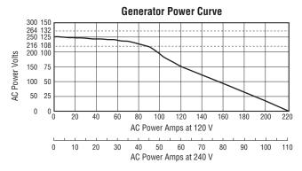
Tools and motors are designed to operate within 10 percent of 120/240 V. The power generator of the Bobcat provides strong power while keeping the voltage within 10 percent of 120/240 V. **This increases tool/motor performance and life.**
